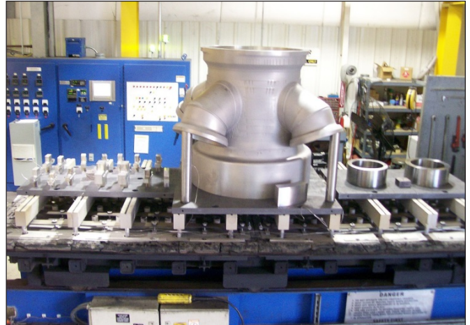
Titanium manifold weldment after vacuum heat treatment.
